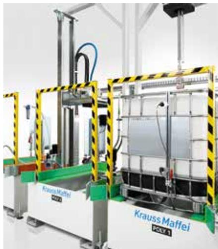
Container station for preconditioning PU components
